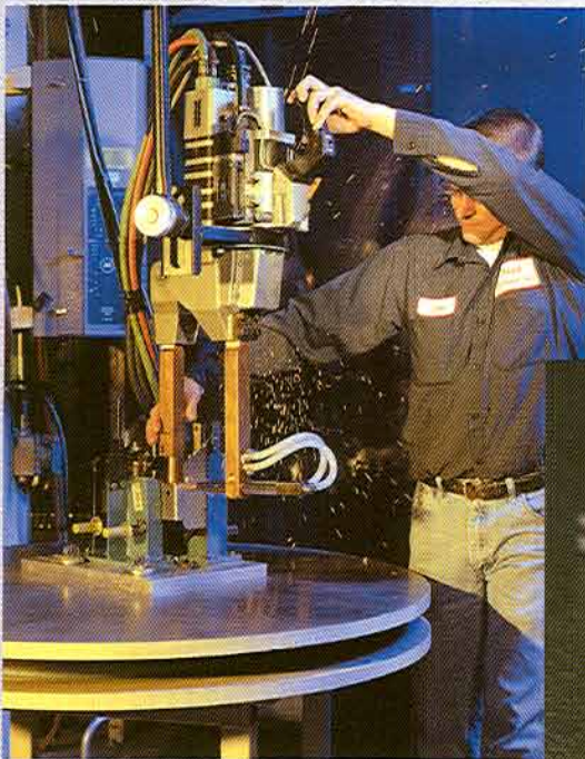
Instrument panel components being assembled using a portable resistance spot welder.
