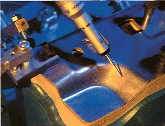
A production check fixture being checked on our Brown & Sharpe coordinate measuring machine.
