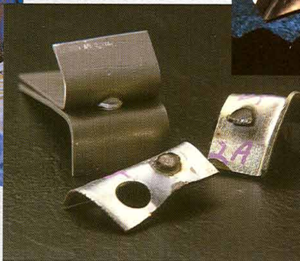
Destructive test samples of a resistance spot weld nugget using the "peel" technique.
